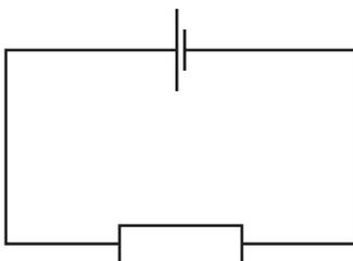
What are the directions of the electron flow and of the conventional current in the **resistor**?
